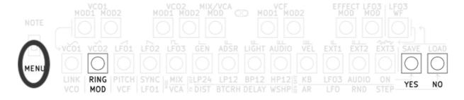
When the ring modulator is enable, the VCO2 signal is replace with the ring modulator signal.
