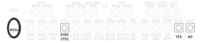
When this option is enable, The LFO1 phase is reset at every GATE signal.
