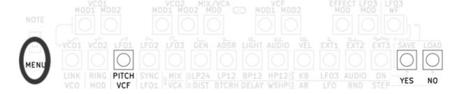
When the filter keyboard tracking is enable, the cut-off frequency of the VCF follow the keyboard pitch.
